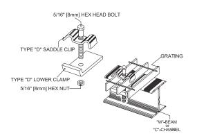
This combination allows for fastening grating without drilling into the supports. The Type D Saddle Clip holds the grating from the top as the bottom clamp is tightened under the flange of the supporting member. Designed for use with Tru-Weld Type 19 and Type 15 bar grating only (in 1/8" and 3/16" bar sizes).
