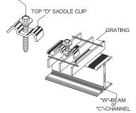
Our most common and cost-effective fastening method. Simply pre-drill a hole into the supporting member and drive in the self-tapping screw. Designed for use with Tru-Weld Type 19 and Type 15 bar grating only (in 1/8" and 3/16" bar sizes).
