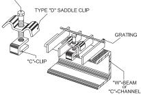
Eliminates the need to drill supports or have access beneath the grating during installation. The C-clamp slides between the bearing bars to clamp the flange of the supporting member and is tightened from above using a hex-driver. For use with Tru-Weld Type 19 and Type 15 bar grating only (in 1/8" and 3/16" bar sizes).
