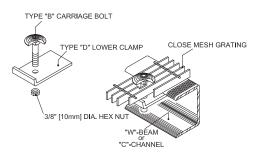
For close mesh Type 11 and Type 9.5 grating, a square collared clamping bolt can be inserted directly between the ends of the bearing bars and fitted through a bottom clamp. The rounded bolt head rests directly on the bearing bars eliminating the need for a top saddle clip.
